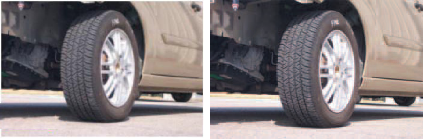
Figure 1.1 – The difference between a correctly inflated tire (LEFT) and one with only 70% pressure (RIGHT) is difficult for a typical driver to see.
