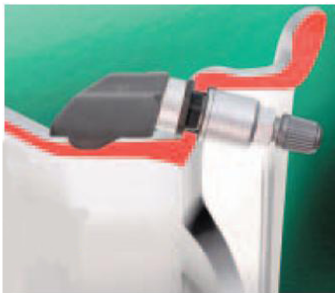
Figure 1.2 – BERU's sensor module mounts inside the tire on the valve stem
