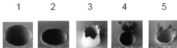
Figure 1.7. Burr classification according to (Berger 2002) [3]
