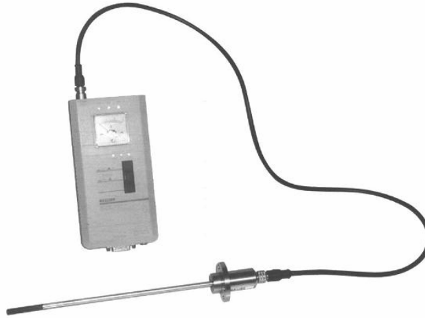
Figure 3.1. Inductive Sensor and BIG P A065E Device [7]
